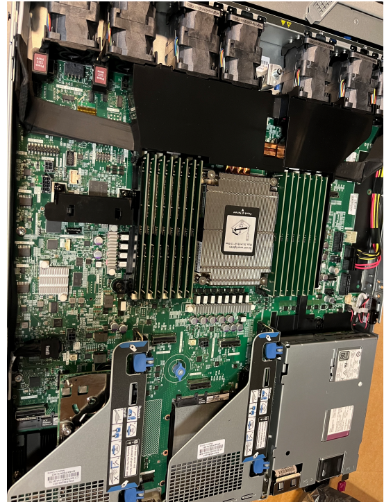
(b) RL300 w/ Slingshot adapter installed.
